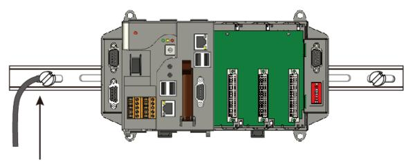
Connect the ground lead to the ground screw
