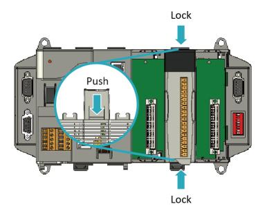
Step 3: Attach field wiring using the terminal block, and then insert the terminal block
