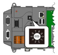
Rotary Switch is an operating mode selector that provides functions to configure with the selection of operating mode and authorization control.
