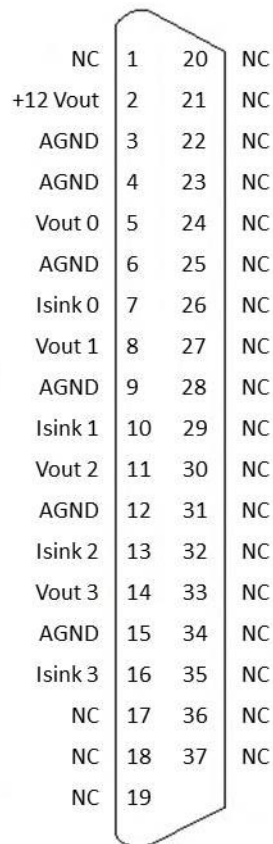
Figure 3.4 PCI-1720U Pin Assignments
