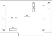
Card connector, jumper and switch locations
