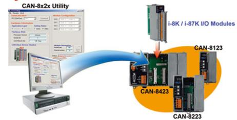
CAN-8x23 main unit can be plugged in the I-8K/I-87K IO modules to create a customized CANopen slave device and application. The CAN-8x23 Utility tool can configure the IO connection path, assembly and application objects information and create the EDS file of the device.
