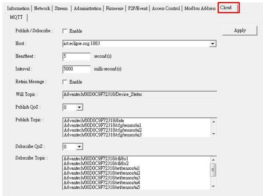
Users could set up the broker URL or IP address at “Host”. Three public broker sources link are listed in the utility
