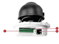
DC 12V Power Input Audio Input / Output Video Output Digital Input / Output DC 5V Power Output
