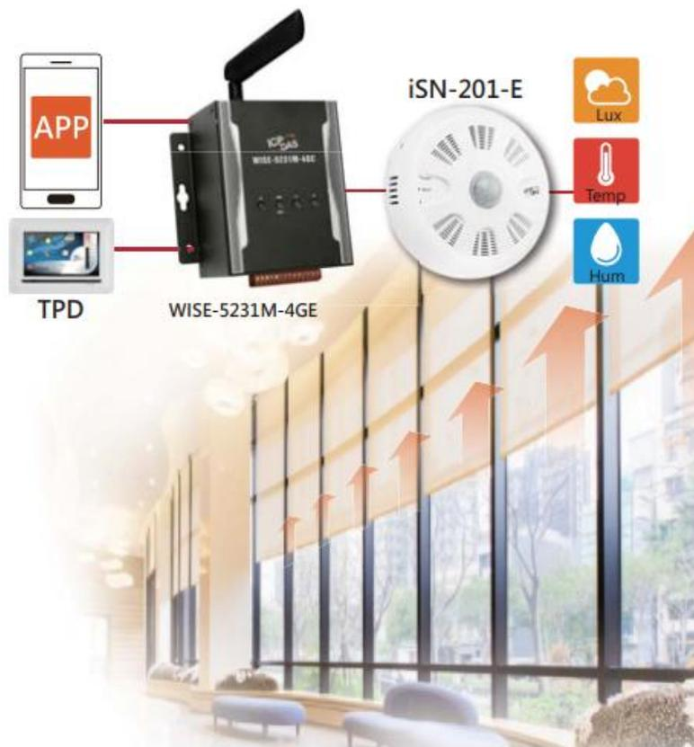
The iSN-201 series contains RS-485, Ethernet and PoE communication interfaces, the most common communication interfaces in industrial network. With additional Wi-Fi interface, the iSN-201-WF provides a WLAN connection which makes an easy way to incorporate wireless connectivity into monitoring and control systems.
