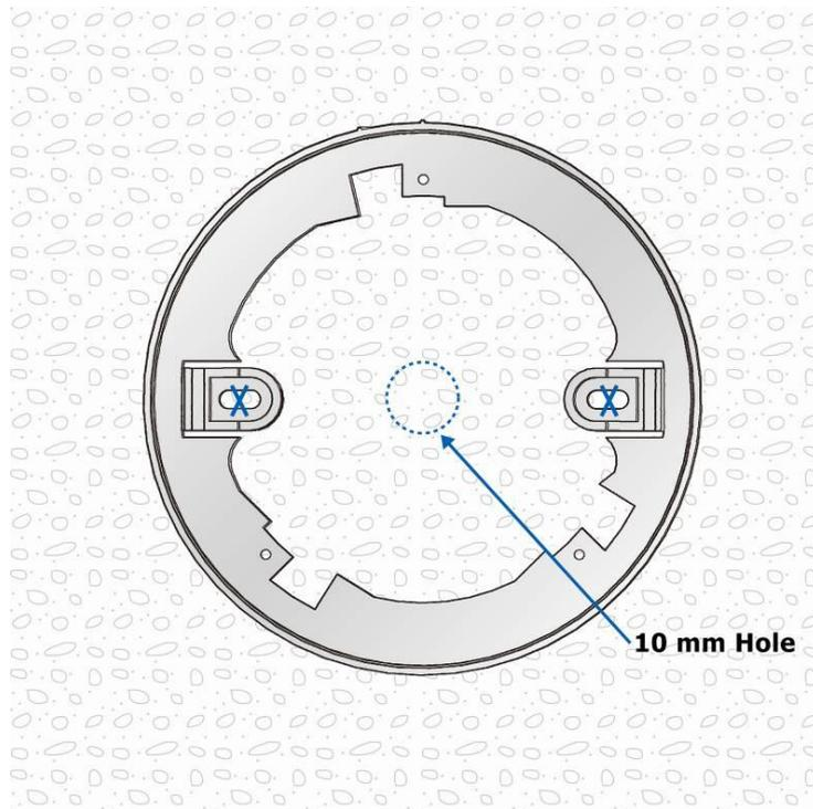
2. Secure the Mounting Plate to the ceiling using the M4x12 drywall screws and the optional octagonal box.
