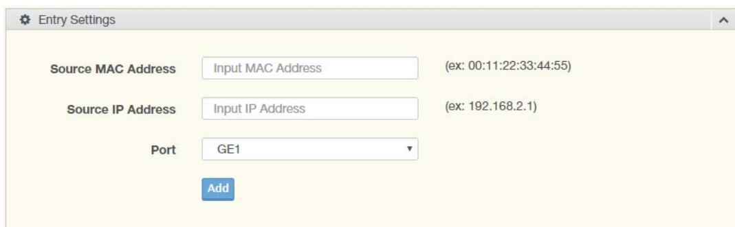
Figure 4.85 Security > IP Source Guard > Entry Settings
