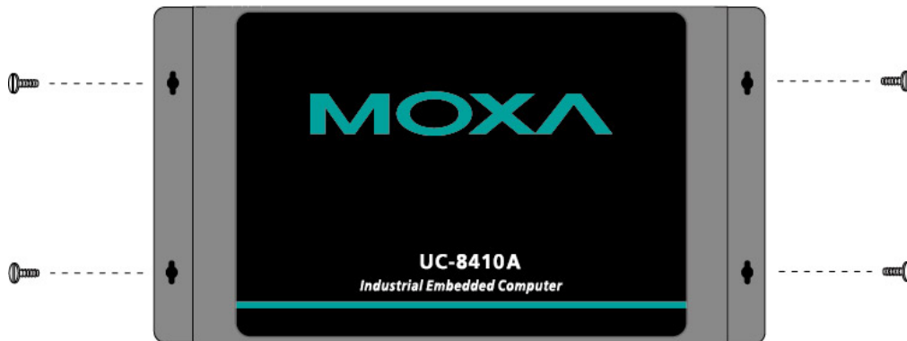
Figure B: UC-8410A Embedded Computer—Wall Mounting Brackets (top view)
