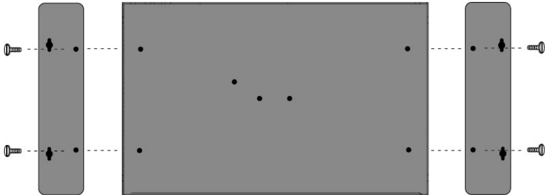
Figure A: UC-8410A Embedded Computer—Wall Mounting Brackets (bottom view)
