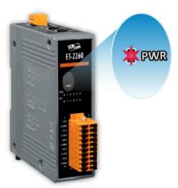
**4** Verify that the **"PWR" LED** indicator on the ET-2260 module is flashing.
