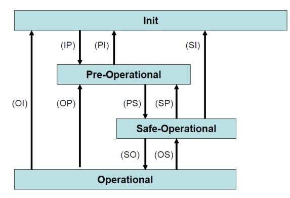
Figure 3: EtherCAT state machine
