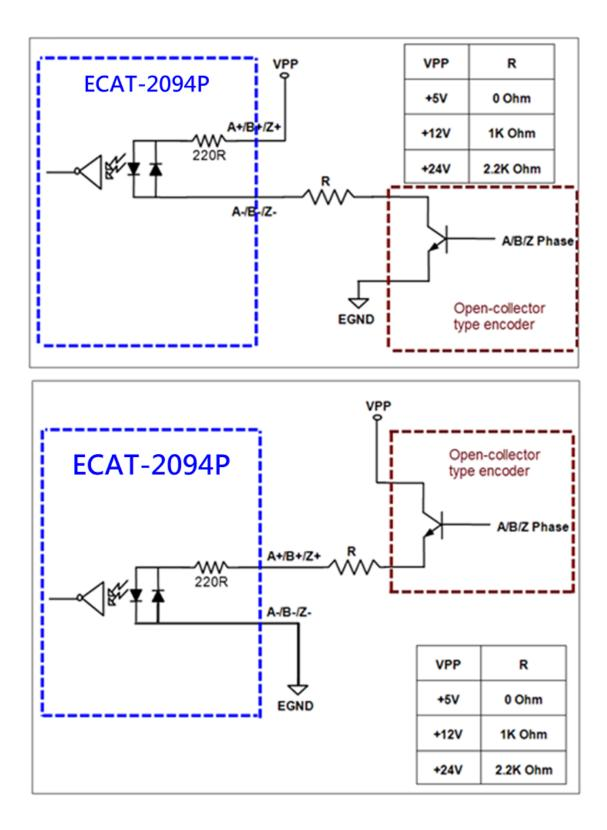
Figure 2: Open collector wiring diagram
