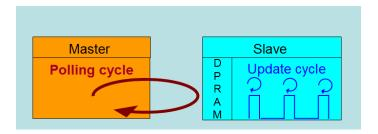
Figure 6: Master-slave cycle in DC mode
