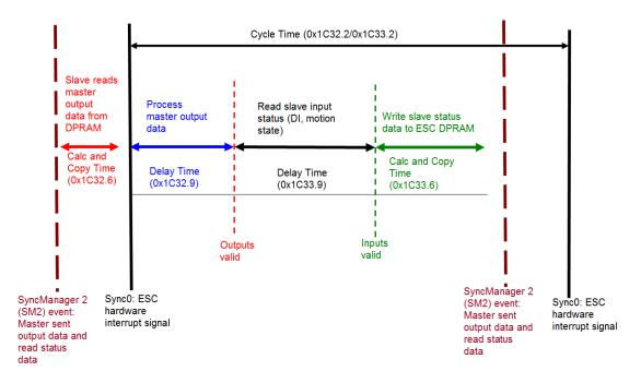
Figure 7: Internal slave processing sequence in DC mode
