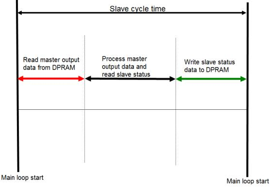
Figure 5: Slave processing sequence in Free-run mode
