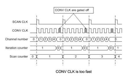
Other scanning procedure applications timing diagram.
