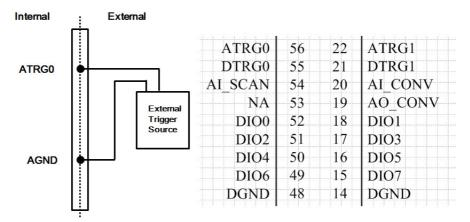
Figure 3.8 External Analog Trigger Source Connection
