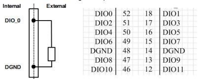
**Figure 3.16 Digital Output Channel Connections**
