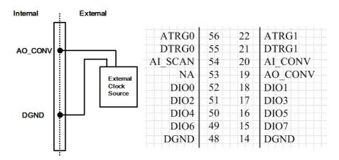
Figure 3.10 External Clock Source Connection
