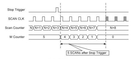
Delay to Stop Trigger (M = 5)
