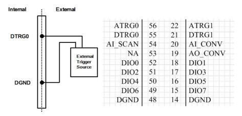
Figure 3.7 External Digital Trigger Source Connection
