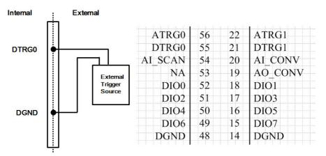
Figure 3.11 External Digital Trigger Source Connection
