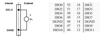
Figure 3.14 Wet signal connection of digital input
