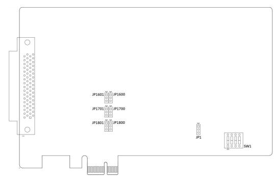
**Figure 3.1 Connector and Switch Locations**
