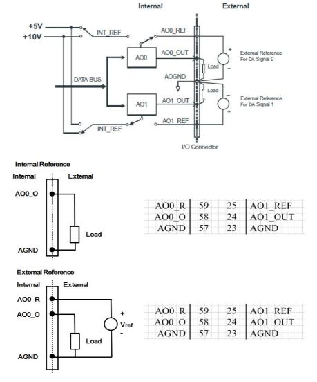
**Figure 3.9 Analog Output Connections**
