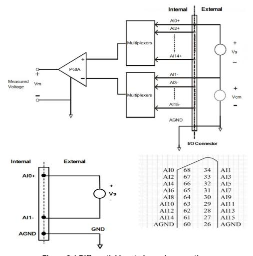
Figure 3.4 Differential input channel connections
