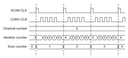
Multiple Iteration timing with fixed channel
