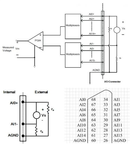
Figure 3.5 Differential input channel connection - floating signal source
