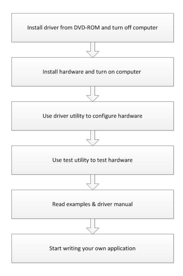
**Figure 1.1 Installation Flow Chart**
