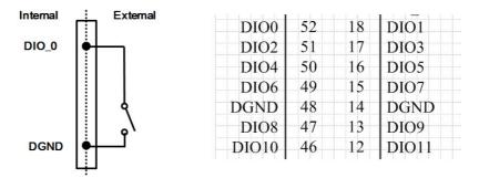
Figure 3.15 Dry signal connection of digital input
