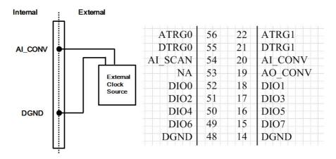
**Figure 3.6 External Clock Source Connection**
