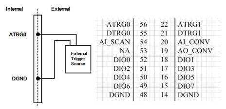
Figure 3.12 External Analog Trigger Source Connection
