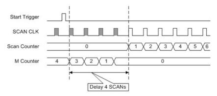
Delay to Start Trigger (M = 4)
