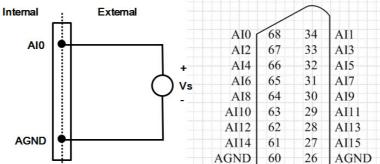
Figure 3.3 Single-ended input channel connections
