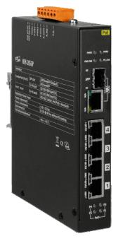
The NSM-205GP is 5-port unmanaged full Gigabit Ethernet switch supporting Power-over-Ethernet on ports 1 to 4. The switch is classified as power source equipment (PSE), and when used in this way, the NSM-205GP switch enable centralization of the power supply, providing up to 30 watts. The NSM-205GP can be used to power IEEE 802.3af/at standard devices (PD).
