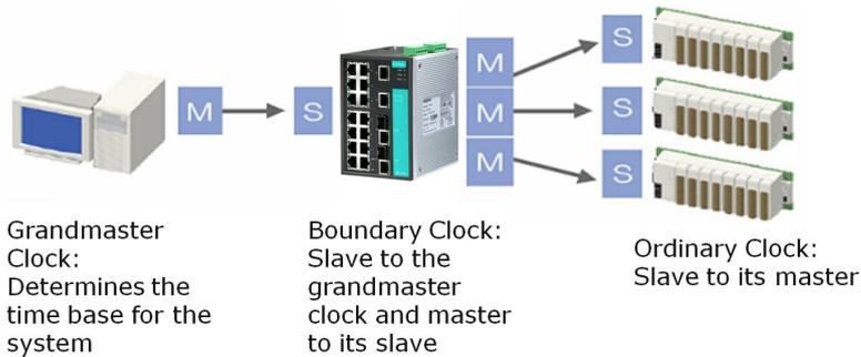
1. The **Boundary Clock and Transparent Clock** functionalities defined by IEEE 1588 must be implemented in the switch.
