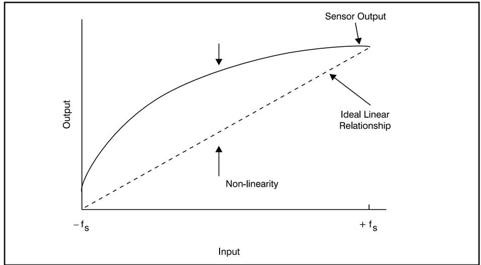
Figure 3. Sensor Terminal-Based Linearity
