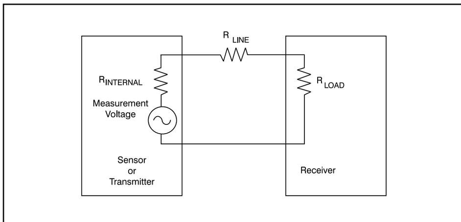
Figure 21. Typical Voltage Loop
