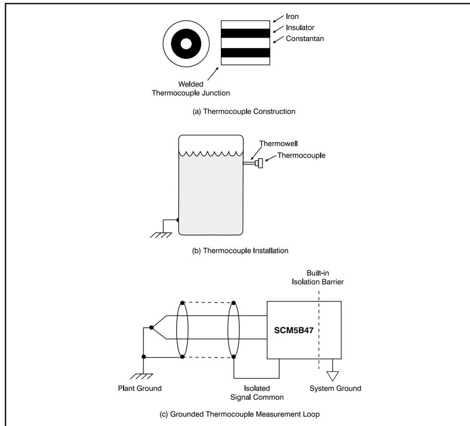
Figure 33. Grounded Thermocouple Application
