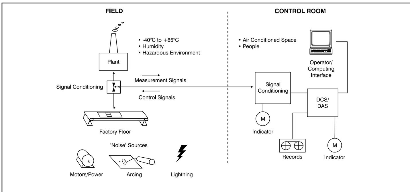
Figure 2. Control and Field Conditions — Industrial Measurement Environment
