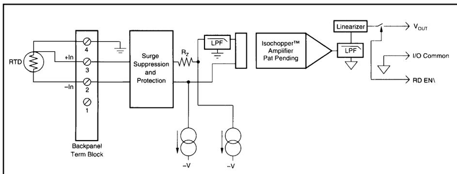
Figure 9. Three-Wire RTD Connection (SCM5B34)
