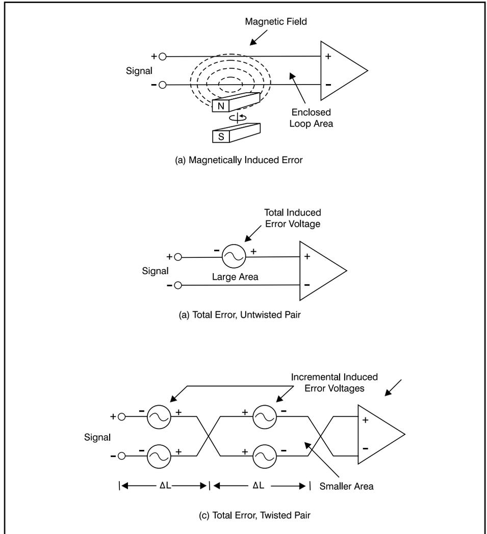
Figure 30. Twisted Wire Pairs Reduce Magnetically Induced Errors
