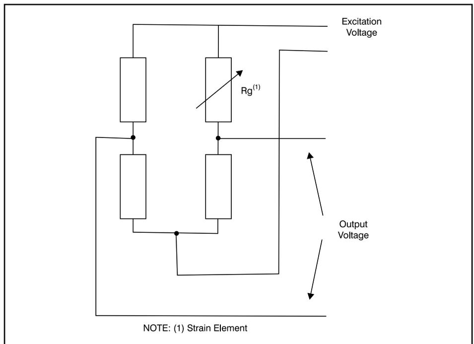
Figure 15. Quarter Bridge Strain Gage
