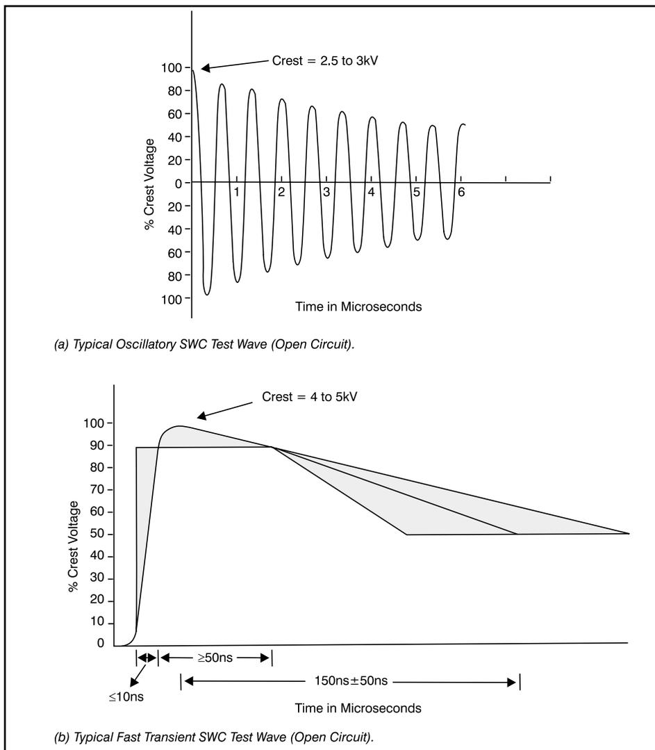
Figure 26. ANSI/IEEE C37.90.1-1989 Test Waveforms
