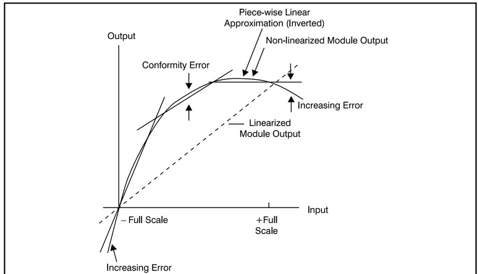
Figure 4. Hardware Piecewise Linearization Using Three Breakpoints
