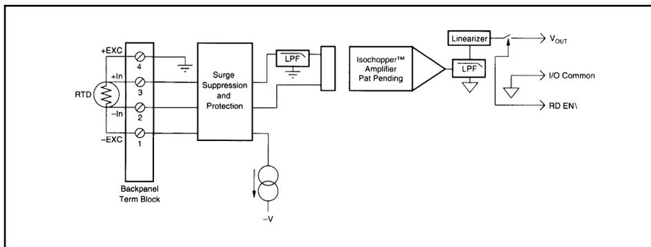
Figure 8. Four-Wire RTD Connection (SCM5B35)
