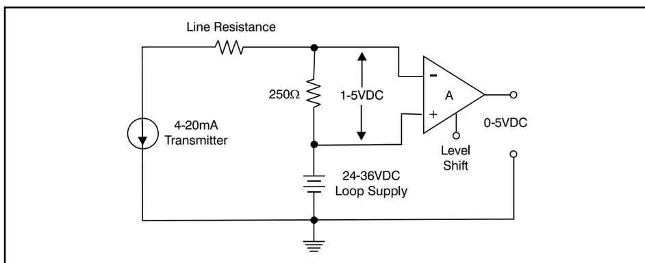
Figure 22. Typical Current Loop
