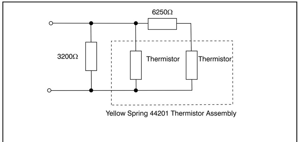
Figure 12. Linear Thermistor Network
