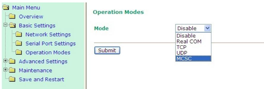
After **MCSC mode** is selected, you will see 2 channels that are ready to be configured. Under the MCSC structure, each channel works independently so you need to configure each channel separately according to your application. Click **Modify** to configure the Channel 1.
