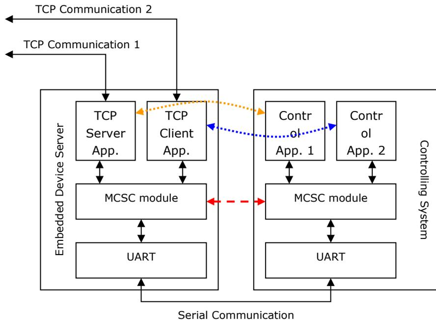
The MCSC module is built into the MiiNePort E1. To enable MCSC, you need to set your MiiNePort E1 serial port operation mode to MCSC mode and then set the channels' operation mode individually according to your application. In addition, you also need to implement the MCSC module in your device's main system.
