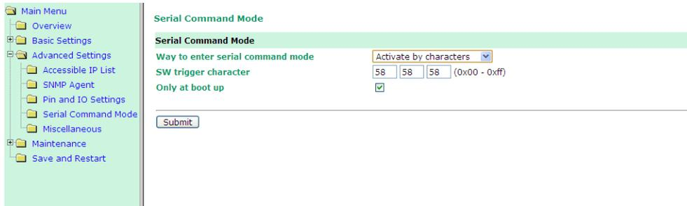
**Activate by break signal:** Break signals are caused by sending continuous Spacing values (no Start or Stop bits). When there is no electricity present on the data circuit, the line is considered to be sending a Break. The Break signal must be of duration longer than the time it takes to send a complete byte plus Start, Stop, and Parity bits.
